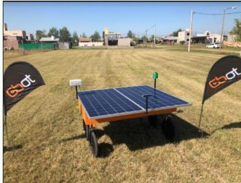
Real-time data collection of field variables, a mobile laboratory unit that fully benefits from its presence in the field to collect data and act on the crop and soil.
